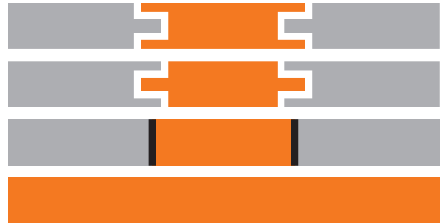
Figure 11: Closed, complete obstruction to the (interim) removal of products or elements.
